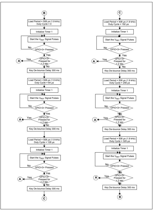
FIGURE C-1: Firmware Flowchart.
