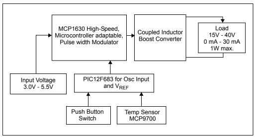
FIGURE 1-1: MCP1630 Coupled Inductor Boost Converter Demo Board Block Diagram.
